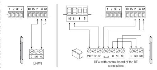
At each opening and closing command, the control board checks the efficacy of the safety devices (such as, photocells).
