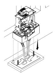
Perforate the cable gland, pass the cables through and fit it into its corresponding housing. Raise the gearmotor by 5 to 10 mm from the plate by turning the threaded feet, to make room for further pinion and rack adjustments.
