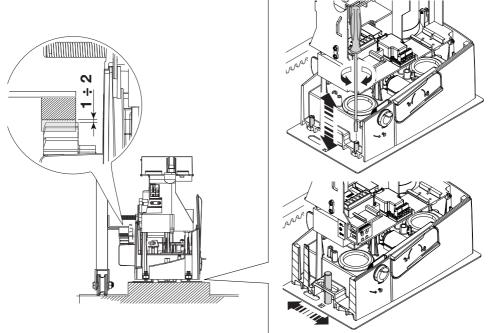
Complete the adjusting, fasten the gearmotor to the plate using the washers and nuts.
