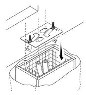
Fill the foundation frame with concrete. The plate must be perfectly level with the bolts which are entirely above surface.
