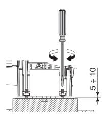
If the rack is already set up, the next step should be to adjust the rack-and-pinion coupling distance, otherwise, fasten it:
